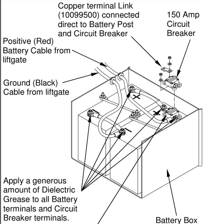
**NOTE:** Circuit Breaker is to rest solidly on the battery to prevent vibration during transit.
