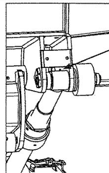
**Note:** Make sure the grease zerk is facing upwards
