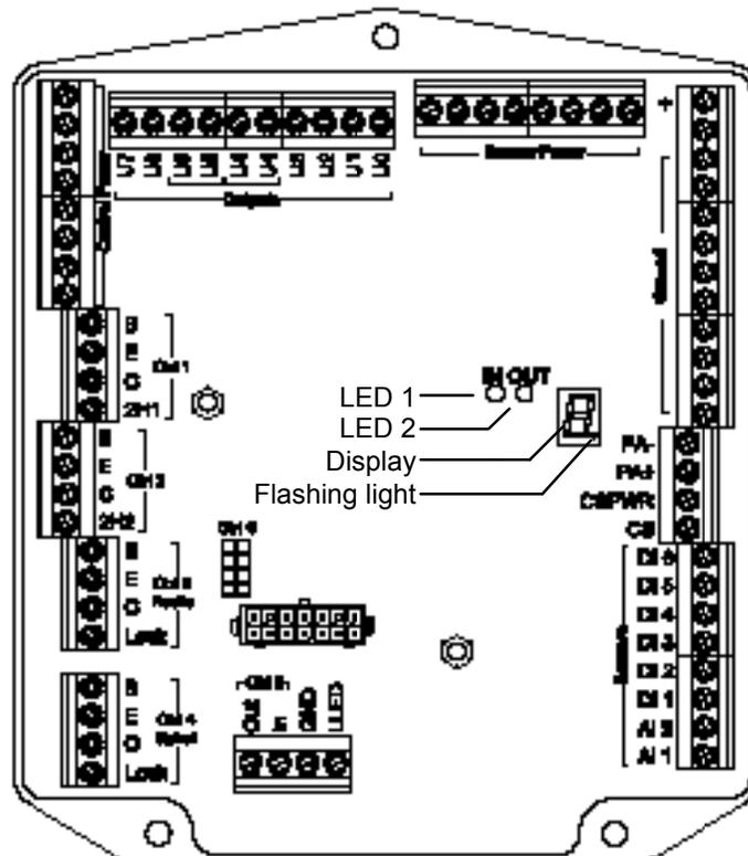
Image 2. The control card is equipped with an alphanumeric display with a flashing light and 2 red LEDs
