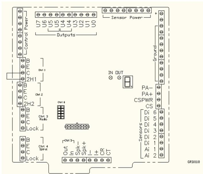
Install the main gate control in control bank 1.
