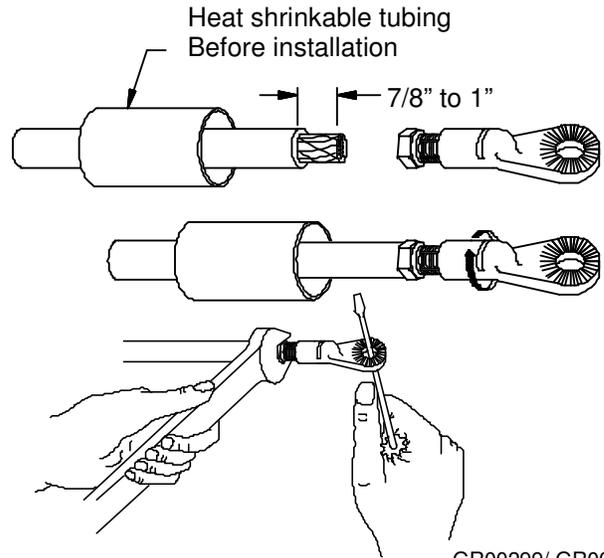
Position heat shrinkable tubing over terminal and end of cable.
