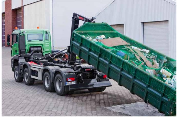
The indicated body lengths consider at present current DIN 30722. Body length can vary in different markets. With the min. body lengths the demountable body can be tilted partly only conditionally. Exact G-Length can be +20mm/-40mm from dimension in the table depending on the hook height and body standard. Hook height can vary in different markets.
