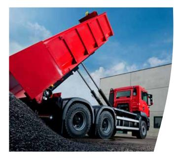
XP Classic hooklifts have a low weight, low installation height and high operating speed. Their optimised construction guarantees a high net payload, as well as fast tipping and body change. High quality top-coat painting at our factory is standard for all MULTILIFT XR and XP models.
