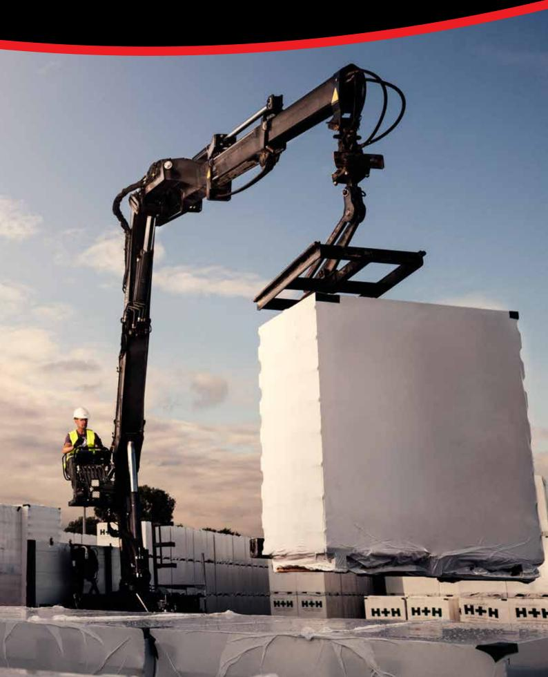
Speed is crucial when handling heavy building materials. The faster the crane, the more goods delivered. The HIAB XS 177K is a powerful and fast worker that offers you unbeatable cost effectiveness and flexibility in materials handling.
