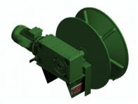
MacGregor electric chain handling winch (ePW) series is designed with variable frequency electric drive. It is a portable unit for easy mounting on board. The advanced drive technology allows safe use of various chain sizes ranging from 76mm diameter up to 160mm diameter by limiting the load on the chain to a preset value. A portable pendant controller is supplied with the winch. Various chain guide rollers and adjustable guide rollers for routing various chain sizes on deck are also available.
