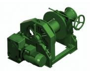
The MacGregor electric tugger winch (eUW) series is designed with line pulls ranging from 5 tonnes to 30 tonnes. For remote operation of drums, hydraulic or pneumatic operated brakes and clutches are available as optional features. A local control is provided next to the winch. Pendant controller or remote control from wheelhouse are also available as options.
