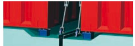
It is, of course, possible to combine the two systems, i.e. external cylinders on the leading pair and internal cylinders on the trailing pairs. Another opportunity to increase the length of the hatch is to insert rolling panels between the folding pairs. They can be towed by the folding cover, thus opening the desired section of the hatch for cargo working. They can also be designed for lifting ashore by container cranes.
