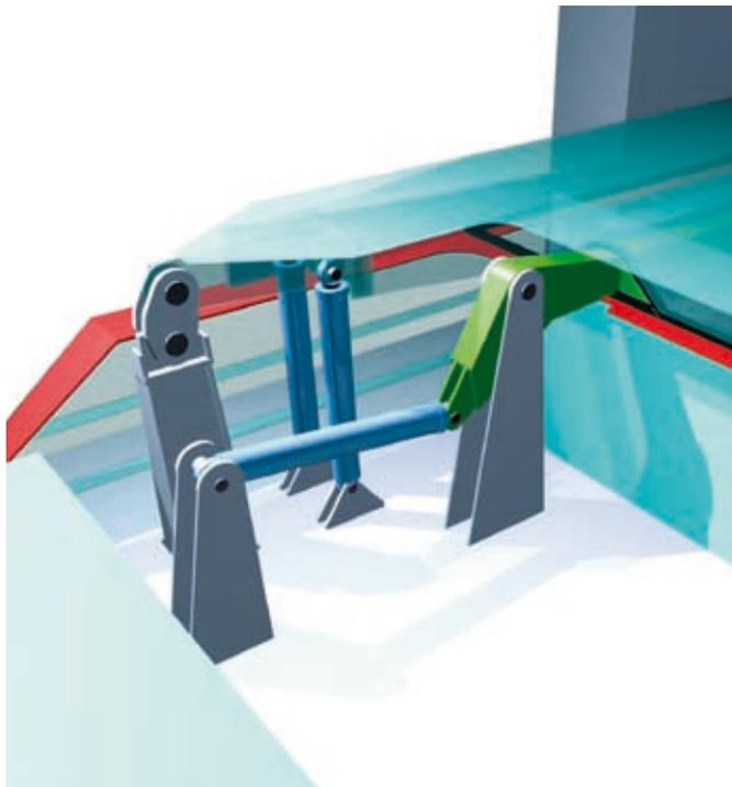
*Bell crank located at transversal coaming*
