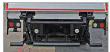
Bumper detail, highlighting the three piece steel bumper
