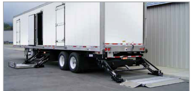
The rear mounted GT and the side load GTSL help to maximize delivery efficiency with two liftgates.
