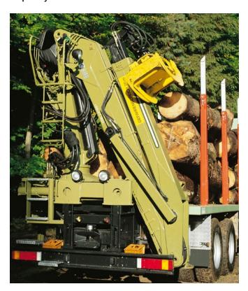
The F165Z/J1620Z is a long-time favourite of the Z-model series. It features a robust, yet easy-to-maintain structure proven in the field. The design allows excellent visibility over the entire loading area. Also, since there are only a few wearing parts, it endures and retains its value over time, like all LOGLIFT and JONSERED forestry cranes.
