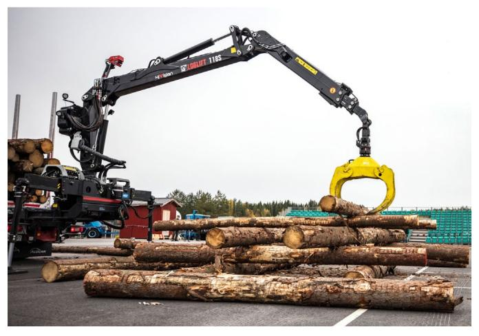
The F118S/J1188S cut-to-length timber-handling crane is available with a choice of several outreaches from 7.9 up to 10.1 metres. It can be fitted with an ergonomic high seat, a cabin with a comfortable, suspended seat or HiVision™. Both the high seat and the cabin offer a selection of options to make your work more
