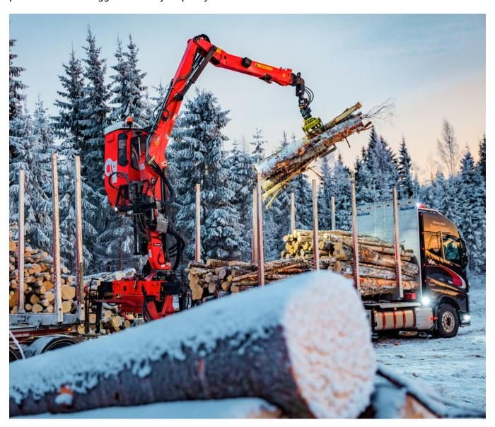
The LOGLIFT F140Z/JONSERED J1400Z is a real power machine. With its 14 tm capacity it is a versatile yet agile companion that will take you through even the toughest jobs in the forest. Its wide array of options will meet the different requirements and preferences. It can be equipped with either High Seat, Cabin or HiVision™. Hydraulic Pilot Control and Hose Protection Link are some of the options.
