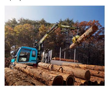
The smallest Z-crane in our product portfolio. Offering an excellent and appreciated combination of lifting capacity and weight. Especially designed for those markets and situations where the allowed vehicle gross weight is limiting your options. Even though the F61Z is our smallest Z-crane, it features all of our standard benefits – durability, reliability, and hydraulic performance.
