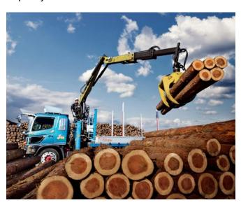
The LOGLIFT F82Z is designed for light trucks. This powerful crane has a long reach, and its ergonomics match that of large cranes. If necessary, it can also be equipped with a telescopic boom. When you need a crane that conserves cargo space and loads cut-to-length timber quickly and accurately, the LOGLIFT F82Z is in a class of its own.
