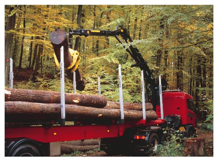
The F265Z/J2640Z is the flagship of the Z-model series, featuring previously unseen lifting capacity and reach in its class. Due to the ingenious design of the long auxiliary cylinder, the performance of the light and compact F265Z/J2640Z is superior compared to other cranes in its class. The F265Z/J2640Z is a good alternative to tree-length cranes with a straight boom since it does not limit the truck's cab-height or take up valuable cargo space from the timber.
