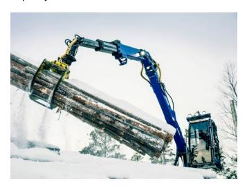
The F108S/J1088S is a real workhorse developed over many years working in the Nordic forests. The F108S/J1088S can be equipped with either a high seat, cabin or  $HiVision^{TM}$  and offers a range of options. Double rack slewing with end dampers offers strong and smooth movement throughout the workday.
