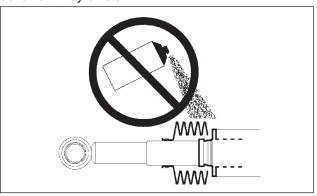
Hydraulic hoses or cables must not be painted, the paint's solvent can damage the hose's/cables rubber compound and can adversely affect durability.
