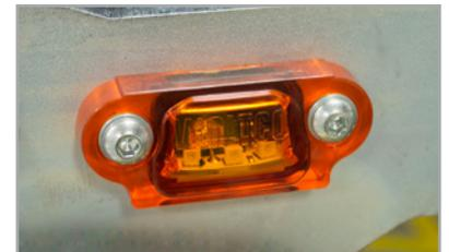
Platform warning lights automatically flash as the platform opens and continue flashing until the platform is closed.
