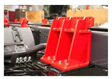
HIAB FRAMEWORKS is a modular system that minimises design work and cuts installation time by 75%.
