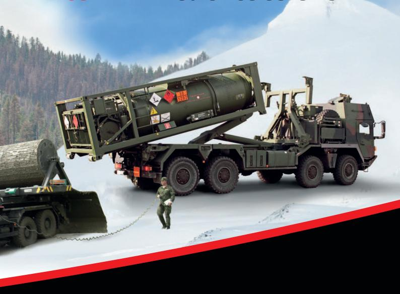
Unloading in the supply area is also enhanced by the system, as loads can be selected at a moment's notice, without the need for mechanical handling equipment and large numbers of labourers. Low mobility transportation can be changed to medium or improved medium mobility category (even high mobility category) if needed, reflecting the locations of the user unit.
