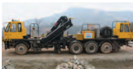
The Hiab cranes were installed on road-rail vehicles along the direction of the chassis frame.
