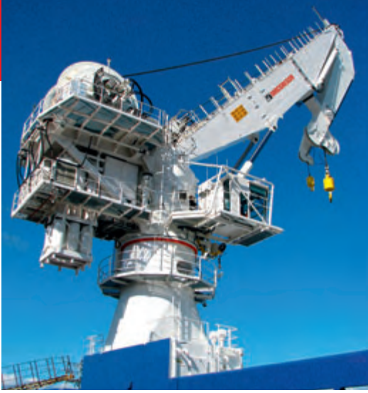
A 150-TONNE MACGREGOR active heave-compensated subsea crane
