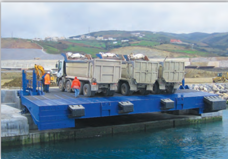
LOAD-TESTING one of the two new RoRo berths delivered by Cargotec at the new Tanger Mediterranean Ferry port
