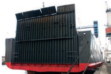
The original stern ramp was removed.
