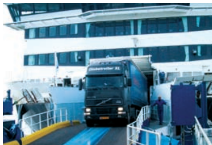
Front bulkhead opened to create a driving passage for trailers was created over the forward mooring deck.
