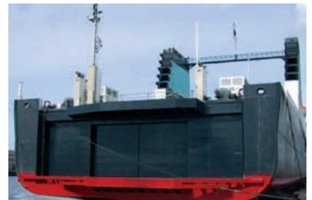
New two-panel side sliding stern door.
