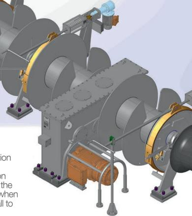
The electrical equipment used for the winches has also been tailored for this particular shipboard application. The programming of the variable frequency drive had to be specially developed in cooperation with the supplier, for example while MacGregor also had to develop fail-safe, redundant heating systems to ensure that all equipment functions could be guaranteed to work under any circumstances.
