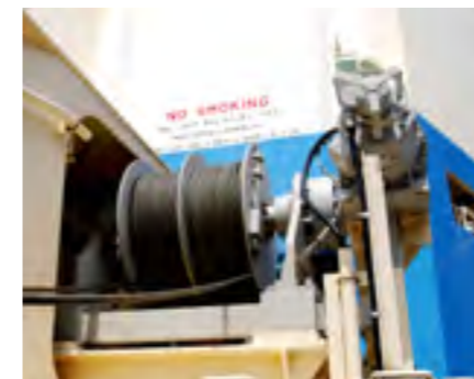
Electrically-driven MacGregor stern quarter ramps and side ramps are operated by electric winches with power feedback system.
