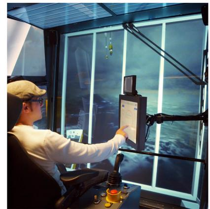
The simulator can be built and delivered as a fixed station at client's facility or as a mobile unit, contained in a 20-ft container with a full crane cabin environment, trainer station, cooling system and a viewing area.
