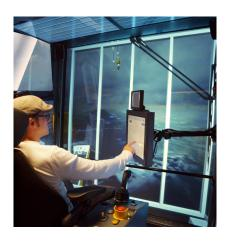
The simulator can be built and delivered as a fixed station at client's facility or as a mobile unit, contained in a 20-ft container with a full crane cabin environment, trainer station, cooling system and a viewing area.
