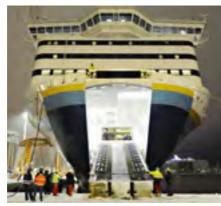
The new bow ramp has a clear driving width of 3,5m and is coated with Bimagrip to prevent vehicles from skidding.
