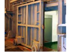
Robust and reliable sliding bulkhead doors have been fitted onboard RFA Argus. They incorporate innovative technology and are developed from proven designs.
