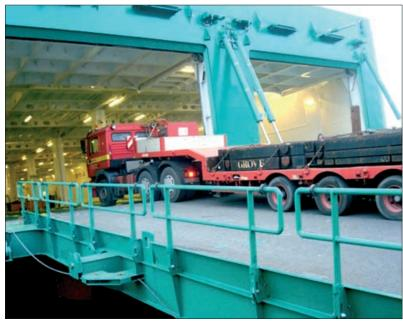
MacGregor's installation team, comprising about 30 people, worked in two-shifts around the clock and completed the installation of two stern ramps on board Tanger Express in just 12 days
