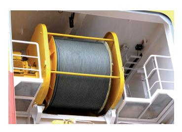
MacGregor winches are supplied with four motors and are redundant in the event of malfunction of one or even two of the motors.
