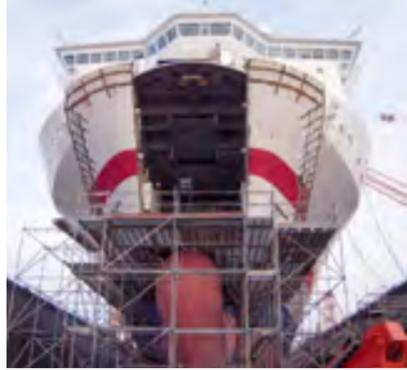
The bow was opened up to arrange new bow doors. A new bow ramp was arranged on main and upper decks.
