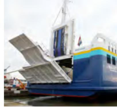
Modification of existing stern ramp, upper stern ramp with slope structure.
