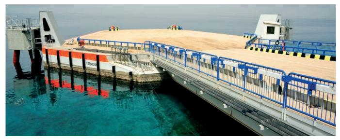
The large hexagonal floating pontoon linkspan was a supply chain challenge. A slipway was constructed at the production site in Croatia to ensure the equipment's safe launch. It was towed across the Mediterranean, through the Suez Canal around Sinai, to its final destination in Agaba Ports, Jordan
