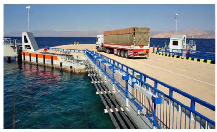
The large hexagonal floating pontoon linkspan was a supply chain challenge. A slipway was constructed at the production site in Croatia to ensure the equipment's safe launch. It was towed across the Mediterranean, through the Suez Canal, around Sinai, to its final destination in Agaba Ports, Jordan.
