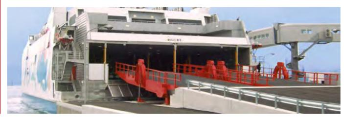
Tailor made MacGregor linkspans for the rampless catamarans are installed in Hakodate and Aomori in Japan. The hydraulically operated linkspans allow quick operation and smooth vehicle transfer across the full breadth of the catamarans.
