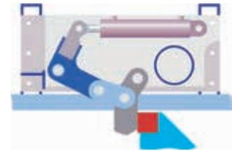
Cleat mechanism for sliding doors
